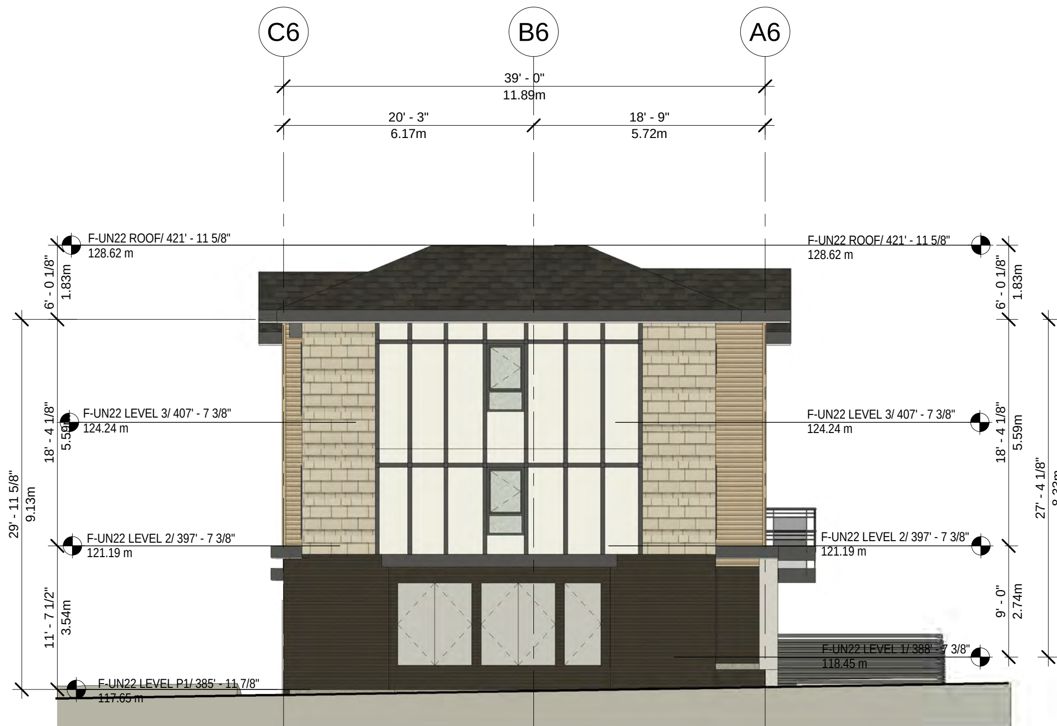
④ Elevation BLD F - South (Left Side) 1/8" = 1'-0"
