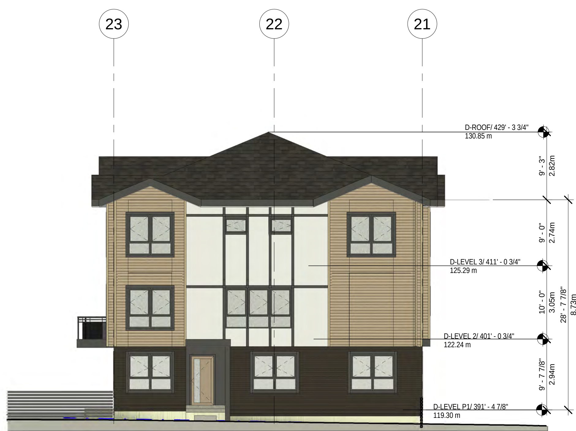
③ Elevation BLD D - East 1/8" = 1'-0"
