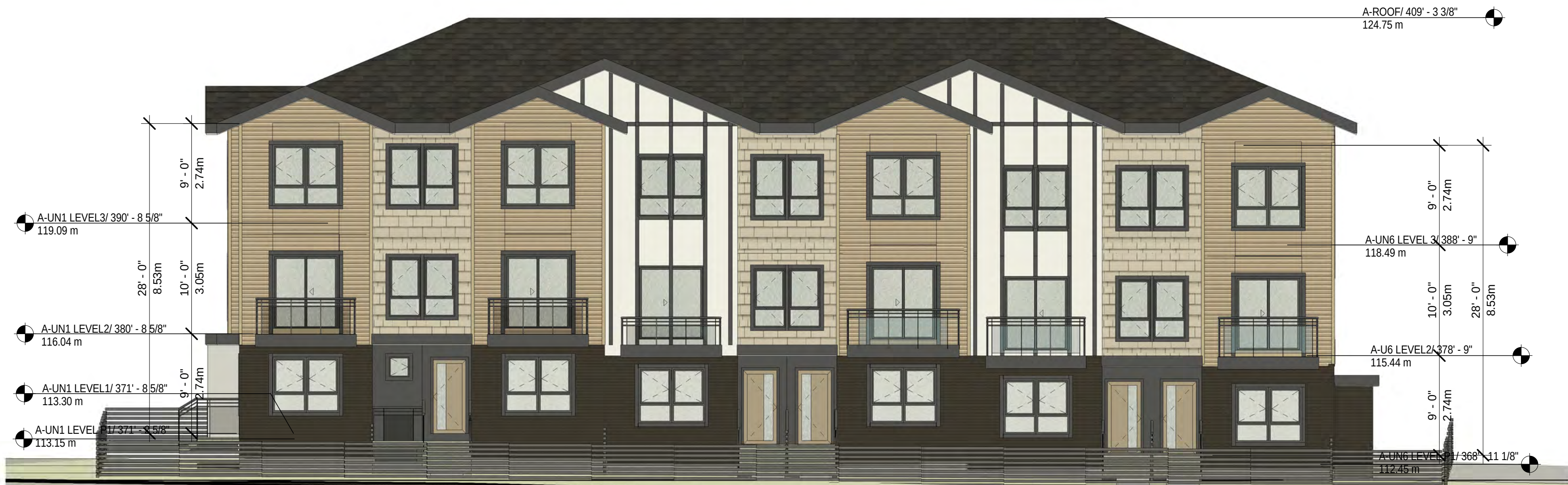
① Elevation BLD A - North (Labieux Rd.) 1/8" = 1'-0"
