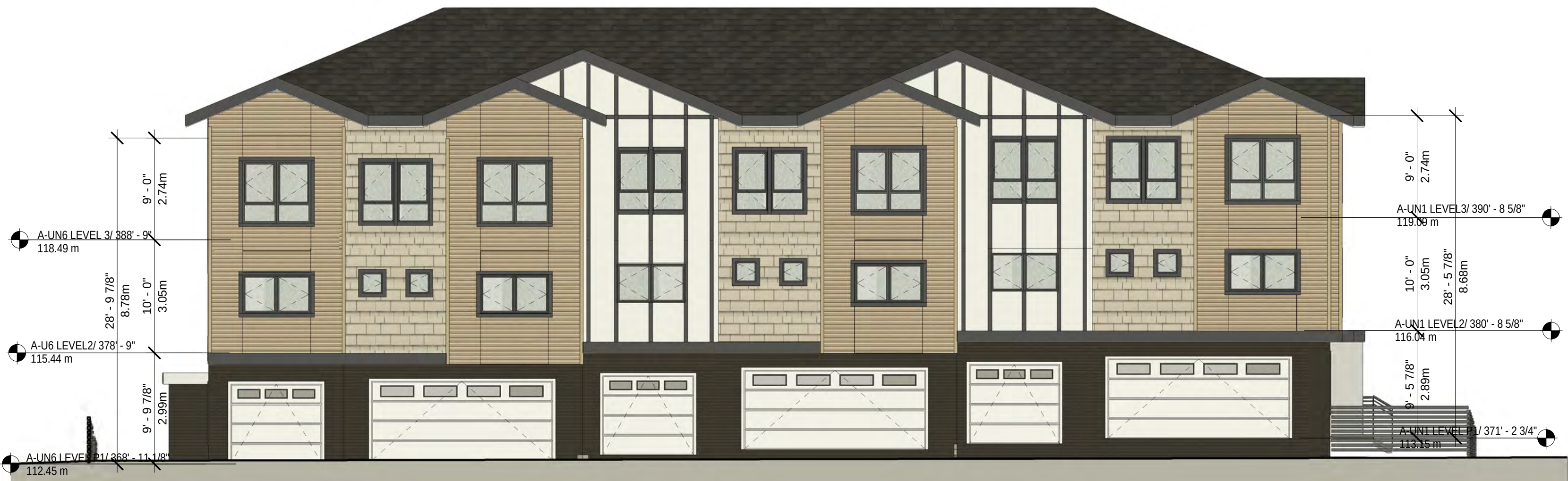
② Elevation BLD A - South (Driveway) 1/8" = 1'-0"
