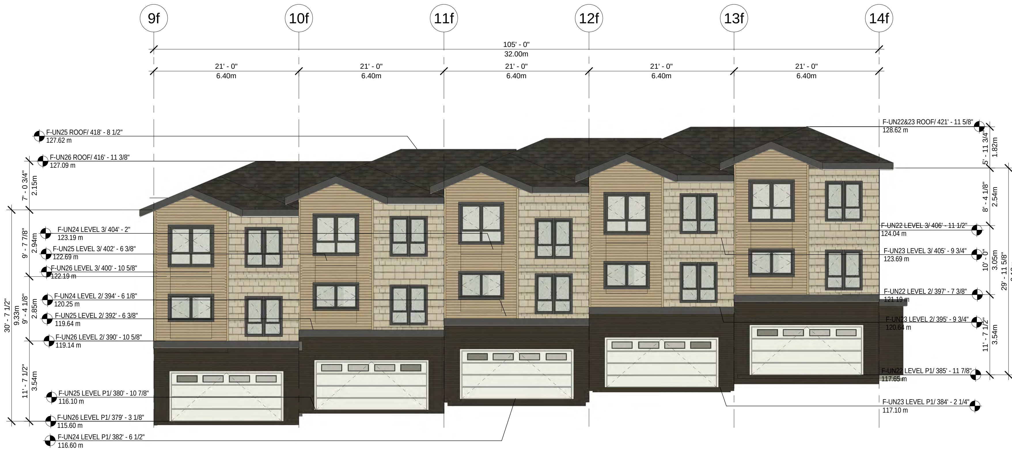
② Elevation BLD F - West (Rear) 1/8" = 1'-0"
